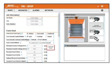
**NOTE:** Antec Toolbox cannot be used to configure FHC's with VFX. Settings must be configured through the Fume Hood Interface.
